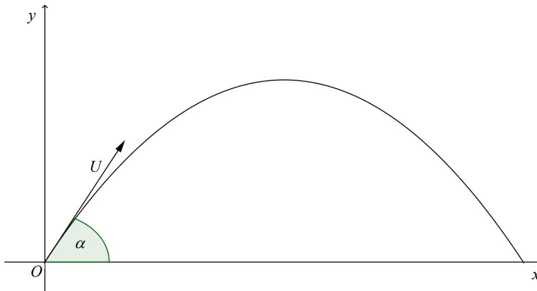
The equations of motion are  $x = Ut \cos \alpha$  and  $y = Ut \sin \alpha - \frac{1}{2}gt^2$ , where  $t$  is time in seconds.
